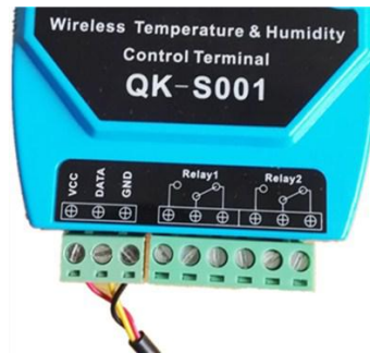
Figure 19 QK-S001T connector
